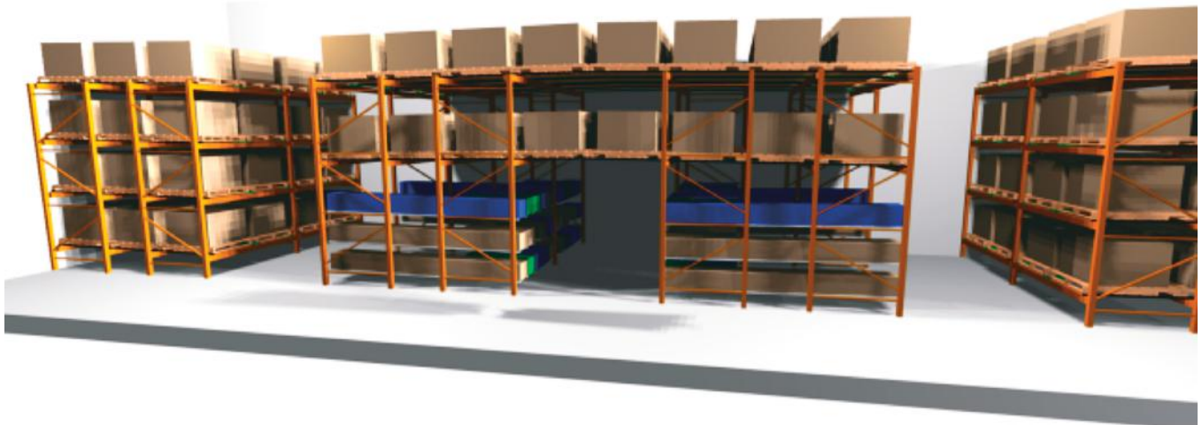
Example Showing Push Back Racking Over Carton Flow Pick Aisle
